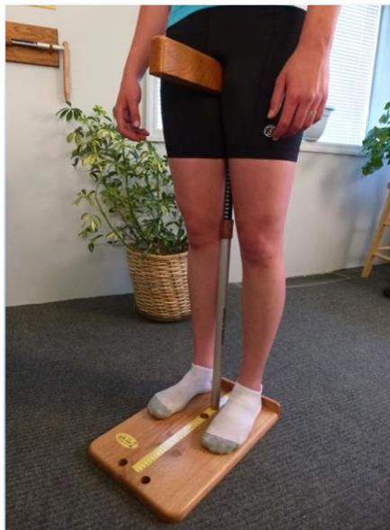
Using the **Inseam Device** with the FIT KIT SYSTEMS **Footboard**:
